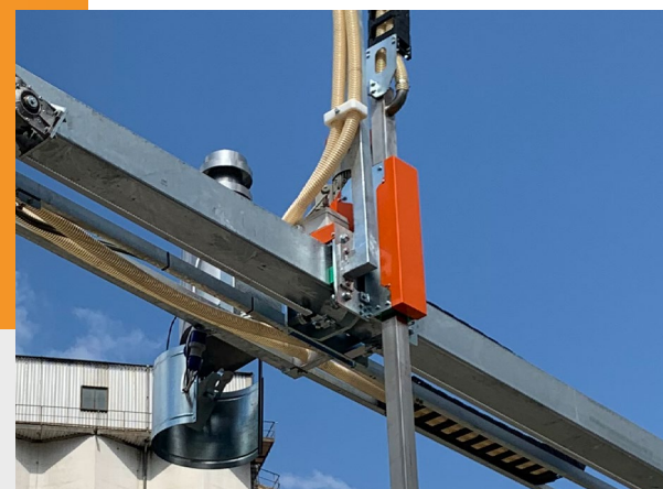
Two-shell square probe with side fastening on the arm for an easy serviceability
