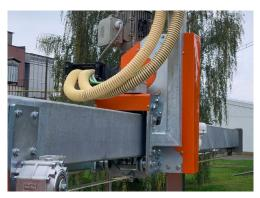
Square doble skin probe with side mounting on the arm for easier serviceability
