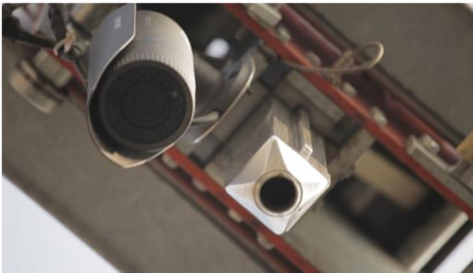
Double-wall sampling probe and camera
